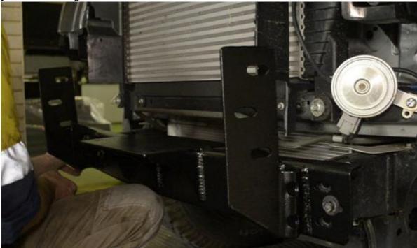
3) We recommend you bolt on cradle finger tight enough so you can move the cradle left to right if you need too. Use 10-15mm foam (clark rubber) or cardboard of equal depth and tape to the bulbar where bar meets guards, use a tape which does not affect the paint. See images below typical image
